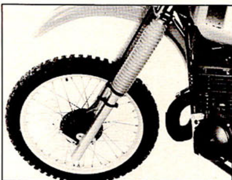
Quick-detach wheel has a strong brake.
