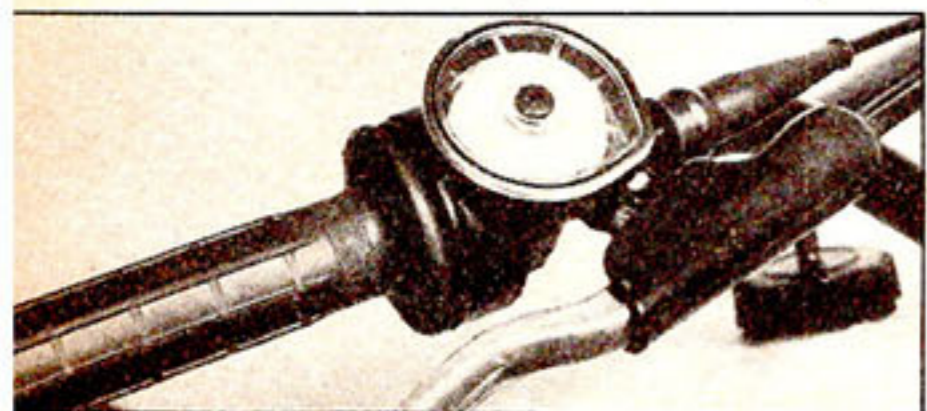
Plastic throttle bevel gears allow cable to run beside handlebar.
