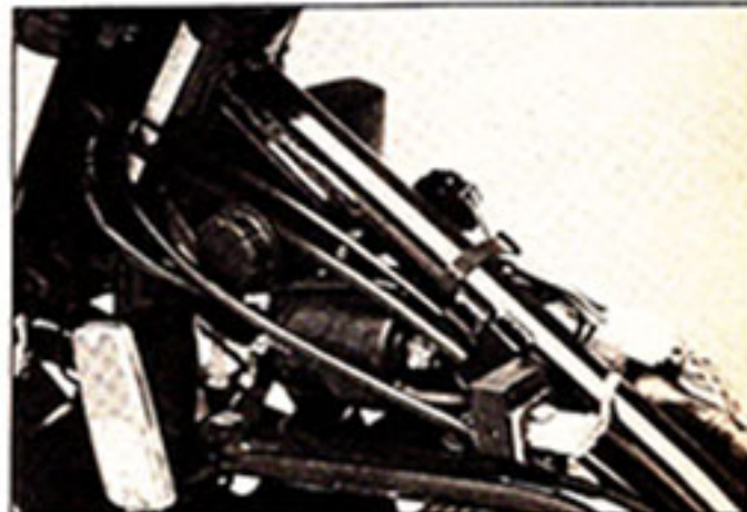
Steering head holds a maze of electric gear from coils to fuel level sender.
