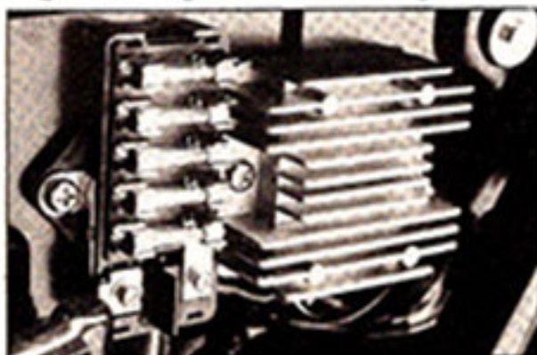
Electrical system has useful provision of a separate accessory power take-off.
