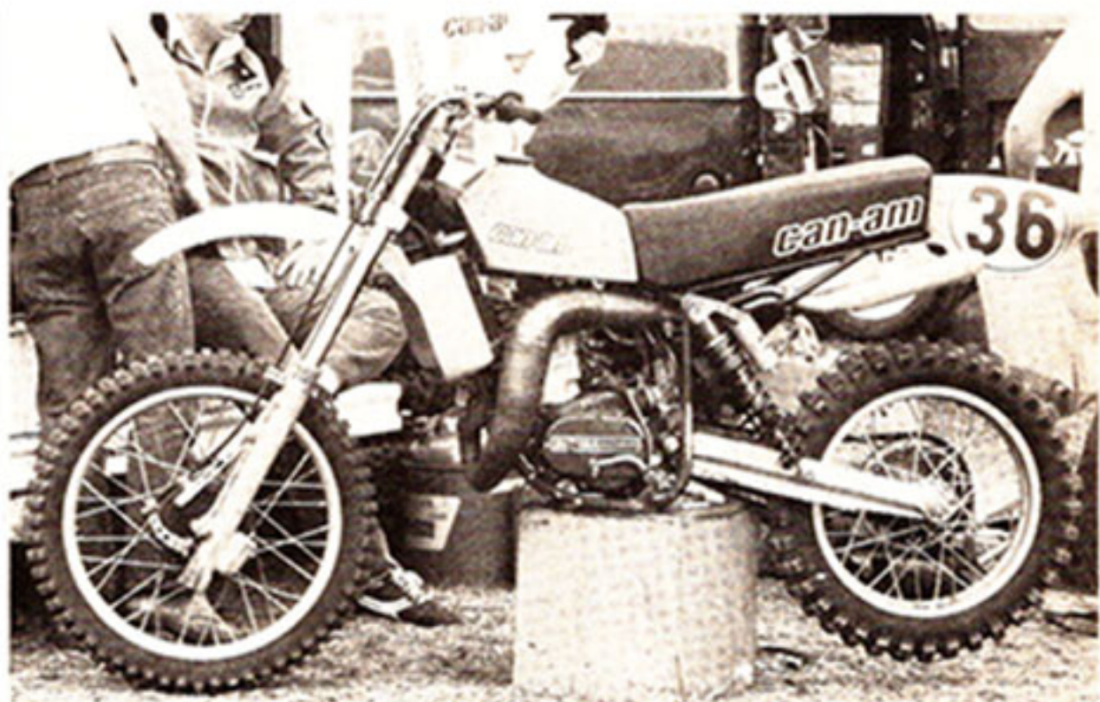
Prototype Can-Am has new fork, engine, frame and swingarm.
