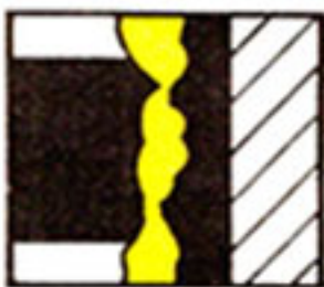
2. High pressures create flash temperatures, heating metals and destroying regular oils.
