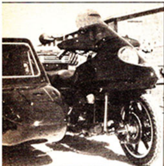
Earles fork lightens sidecar steering.
