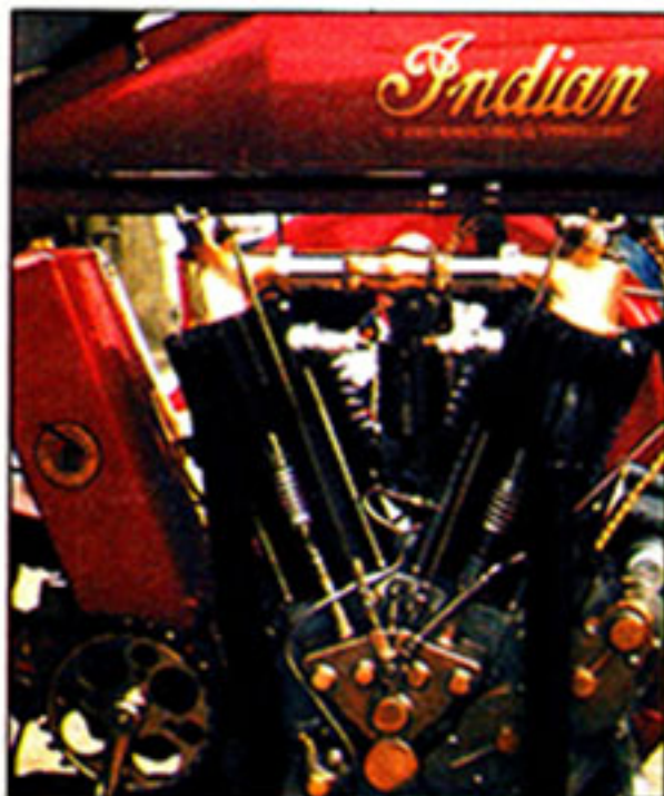
Early Indian was a 1,000 cc moped with overhead inlet valves, side exhausts.
