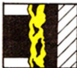
3. Molecular attraction between the hot, bare metals causes them to seize. They weld together and tear. This is friction, the major cause of wear.
