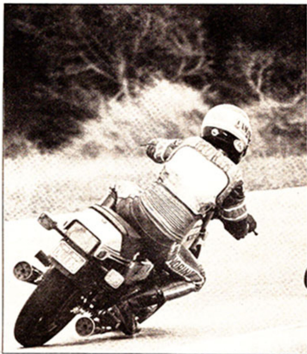
The Suzuki's footpegs and header pipe junctions dragged, but the tires didn't seem to be upset by such shenanigans.
