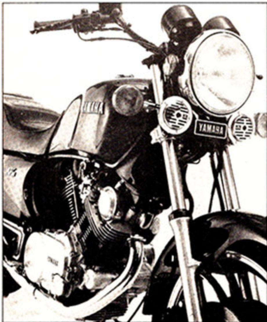
Enormous 200 mm headlight dominates the frontal aspect of the XV920. Fuel tank looks large but holds only 19 litres.
