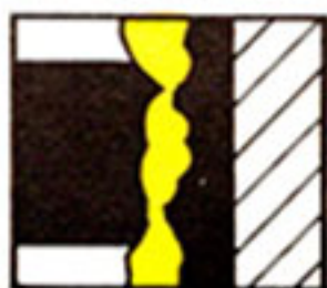
2. High pressures create flash temperatures, heating metals and destroying regular oils.
