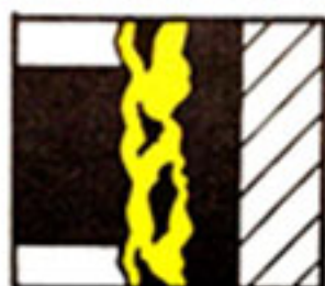
3. Molecular attraction between the hot, bare metals causes them to seize. They weld together and tear. This is friction, the major cause of wear.
