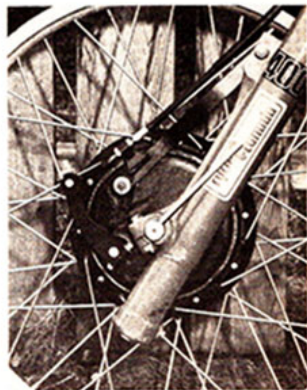
Diamond section aluminum swingarm (left) is a factory option that extends the wheelbase, improving handling and minimizing wheelies. Brake modification (right) improves feel greatly, but doesn't do much for ultimate stopping power.
