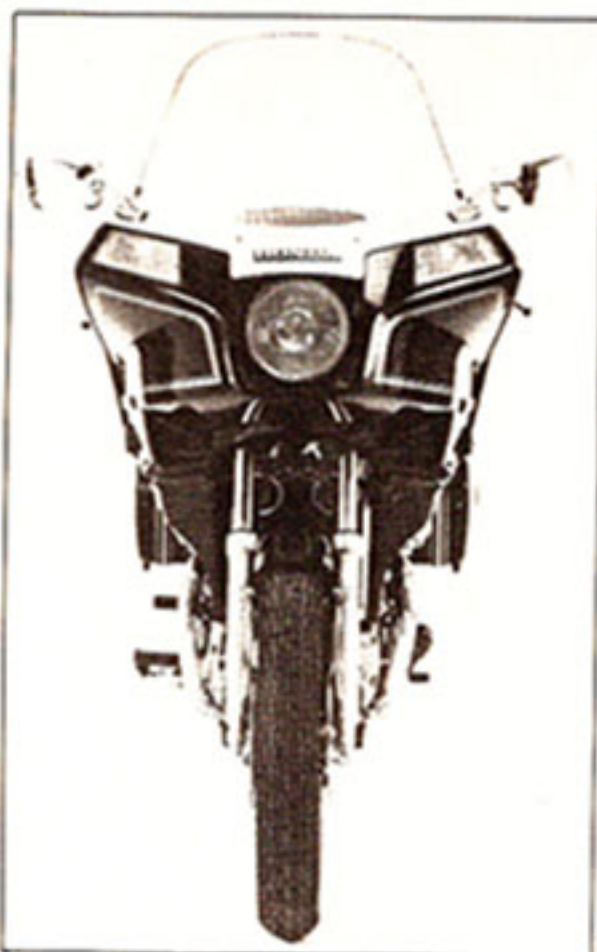
Interstate fairing is one of the best, but the windscreen is too high for most riders.
