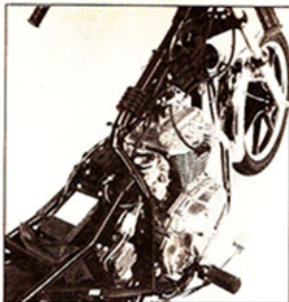
Sturdy frame tubing keeps the 306 cc engine from overpowering the chassis.
