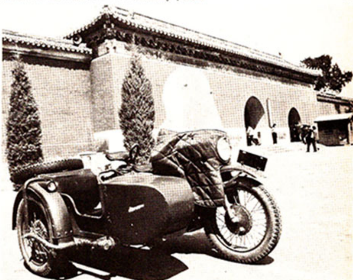
The Yangtze River with sidecar is China's motorcycling workhorse, complete with spare tire, flat twin engine and quilted fairing. It's a copy of a Thirties-era BMW.
