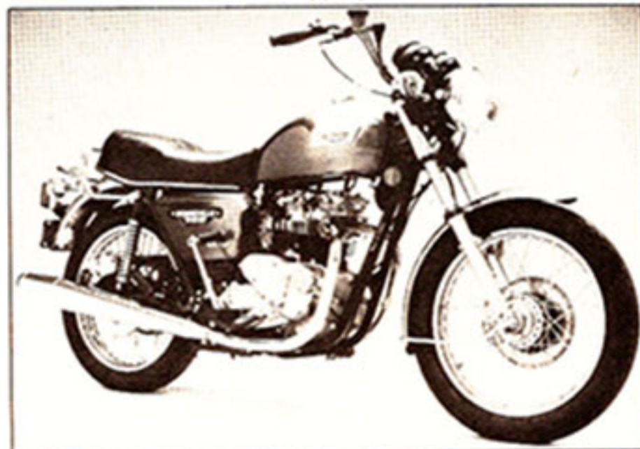
Bulges for electric starter and electronic ignition change the time-honored shape of the Bonneville's timing cover.
