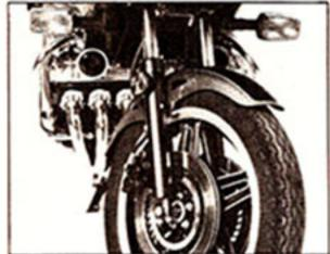
CBX brakes are intricate castinas that let cool air flow radially and axially.
