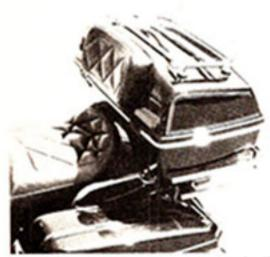
Canadian Cycle Accessories is building a new tour rack for Honda Interstate top boxes. Constructed of heavily chromed tubing, the rack doesn't interfere with normal opening of the box. Suggested retail \$79.95.
