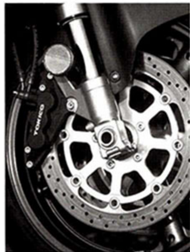
Six-piston calipers squeeze thicker, more heat-resistant discs, offering excellent power and sensitivity.
